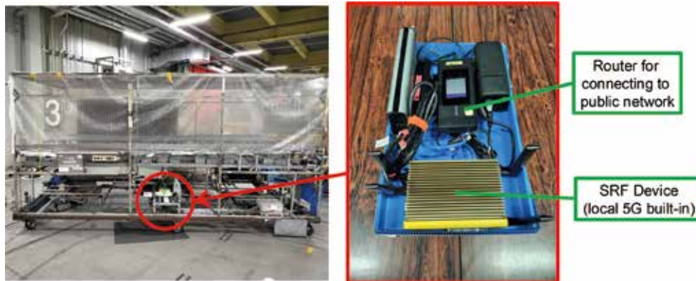
■ Figure 4: Mobile vehicle (AGV) mounting an SRF Device
