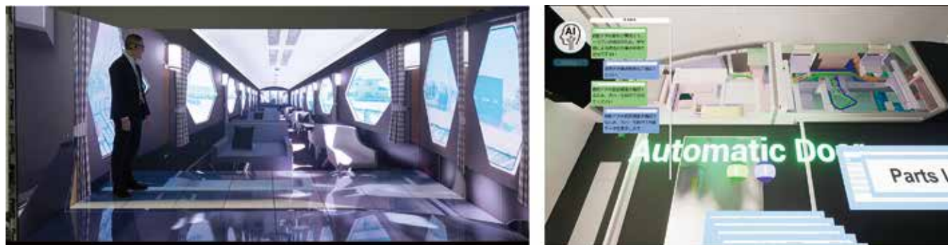
■ Figure 2: Using the rolling-stock metaverse for maintenance. Stakeholders from various departments can participate in the metaverse space and check information linked to work content and location
