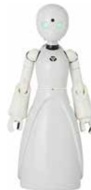
■ Figure 10: OriHime-D operating system
