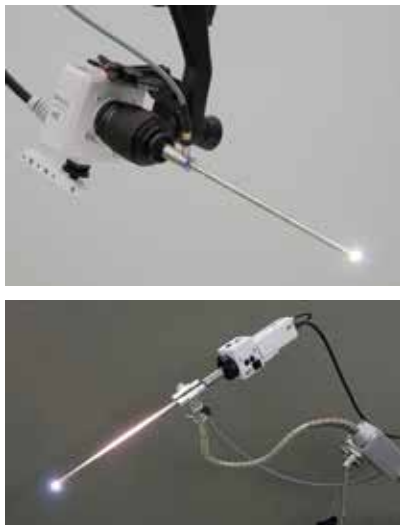
Figure 4: 8K endoscopic camera system Top: Model #1 (2017), Bottom: Model #2 (2020)
