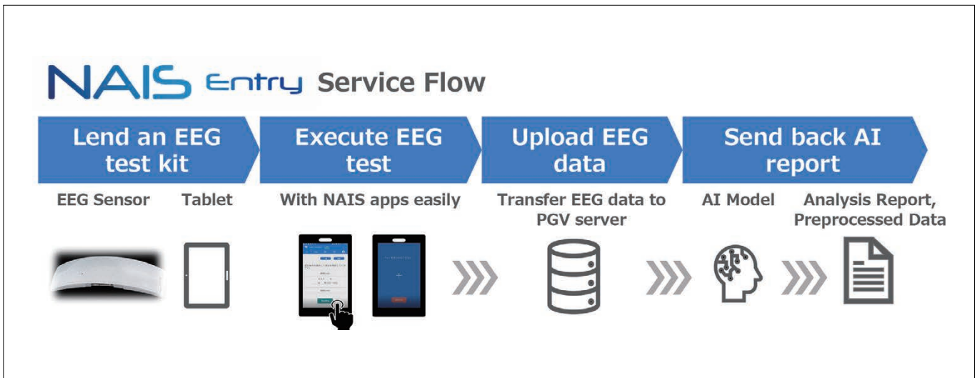
■ Figure 3: NAIS Entry service flow
