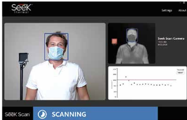
■ Figure 7: Temperature measurement using Seek Thermal
