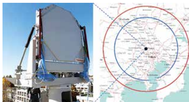
■ Figure 6: Multi-parameter phased array weather radar equipment (left) and observation range (right)
