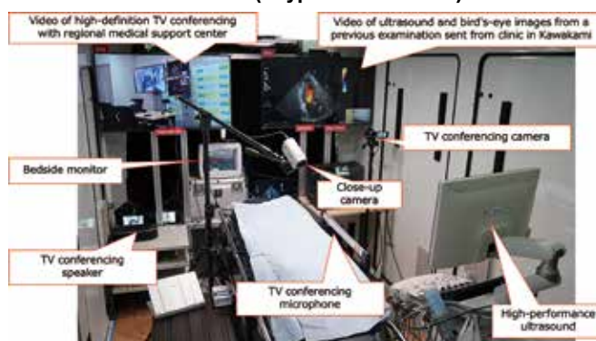
Figure 6: Medical equipment and a bed in a mobile medical unit ("Hyper Doctor Car")
