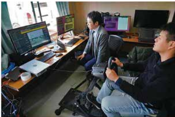
■ Figure 7: Remote operation of abandoned car from a remote surveillance and operation center
