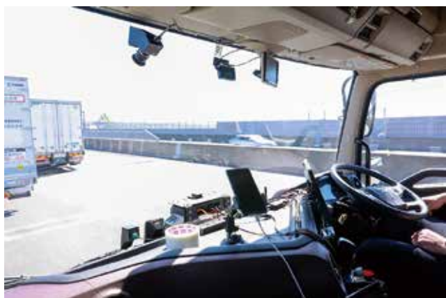
■ Figure 9: Field trial of automated following of a leading vehicle using 5G —automated steering—
