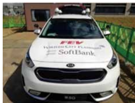
■ Figure 5: Remote-controlled car with onboard 5G user terminal
