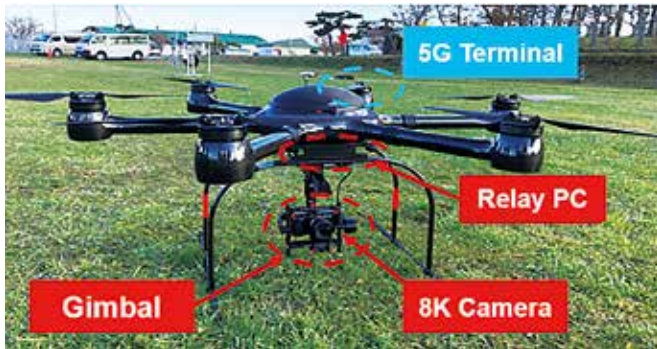
■ Figure 7: Devices mounted on drone
