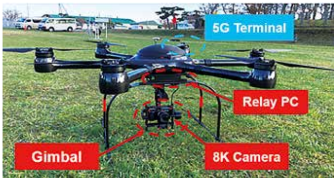
■ Figure 7: Devices mounted on drone
