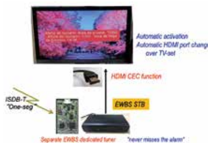
■ Figure 7: Functions of the EWBS STB
