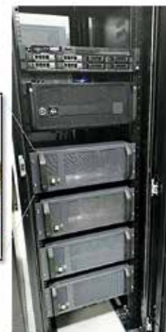
(b) A 100 kbit machine made by connecting 25 FPGAs
