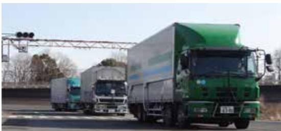
■ Figure 4: Real truck platooning test
