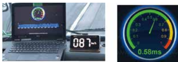
■ Figure 5: V2N low latency communication performance assuming vehicle remote monitoring and control (4.7 GHz band)
