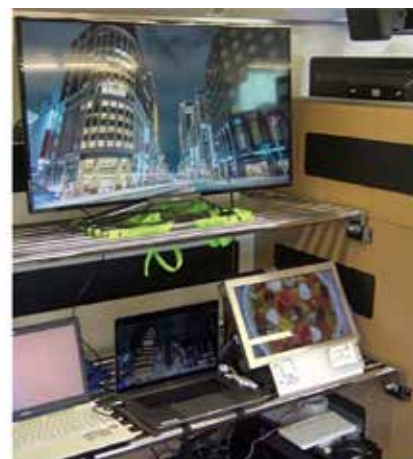
On-train cache server and displays
