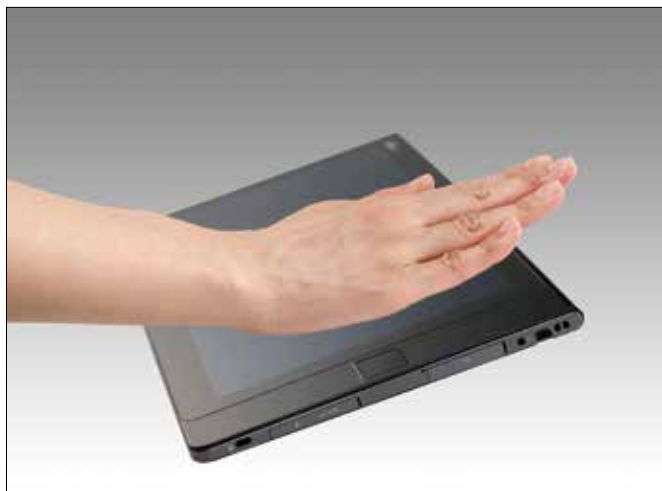
■ Photo 7: Tablet computer with built-in palm vein sensor
