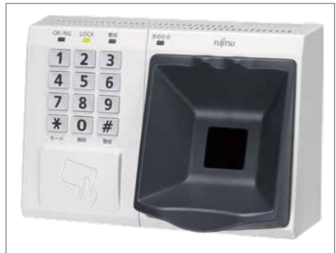
■ Photo 3: Access control panel featuring palm vein authentication
