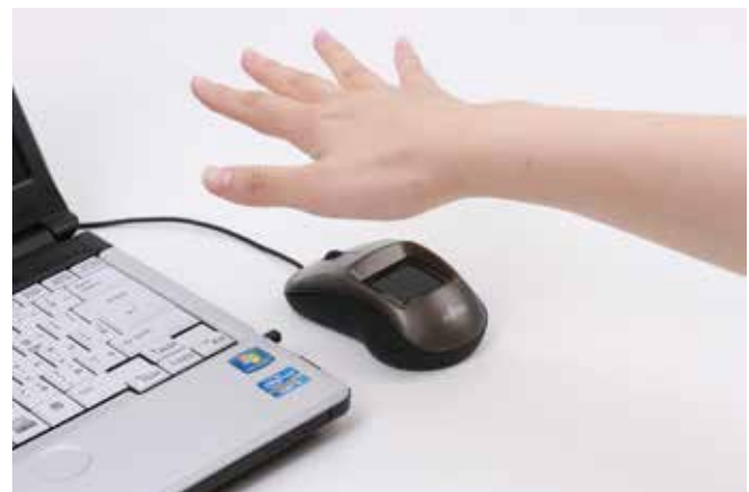
■ Photo 4: Mouse with built-in palm vein authentication sensor
