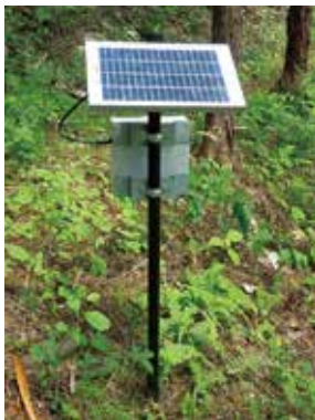
■ Photo 1: Wildlife detection sensor
