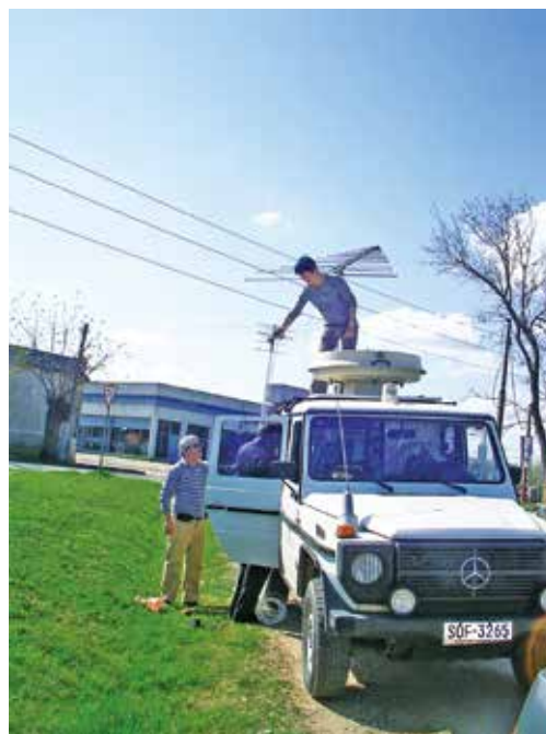
■ Photo 1: Measuring the radio wave characteristics of an area
