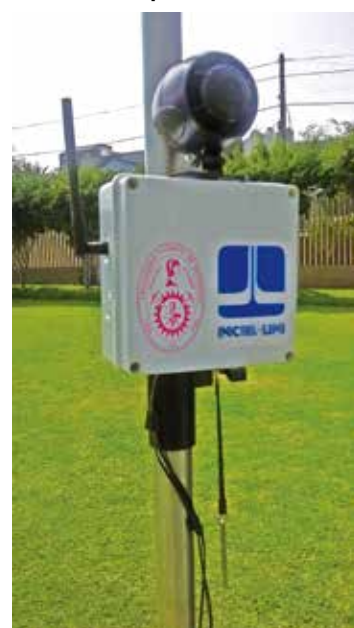
■ Photo 3: EWBS-compatible disaster warning speaker
