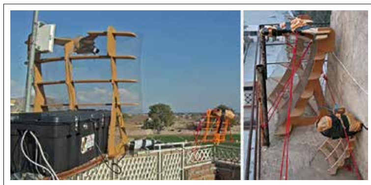
■ Photo 2: A “FabFi” wooden WiFi router produced at the FabLab in Afghanistan
