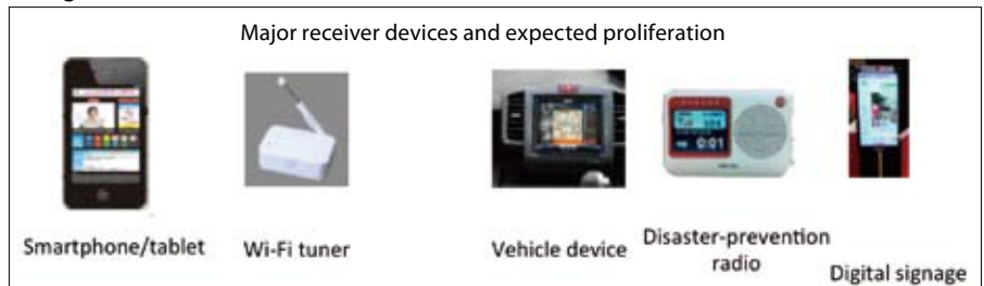
Figure 4: V-Low multimedia broadcast receivers
