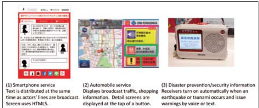
Figure 4: V-Low multimedia broadcast receivers
