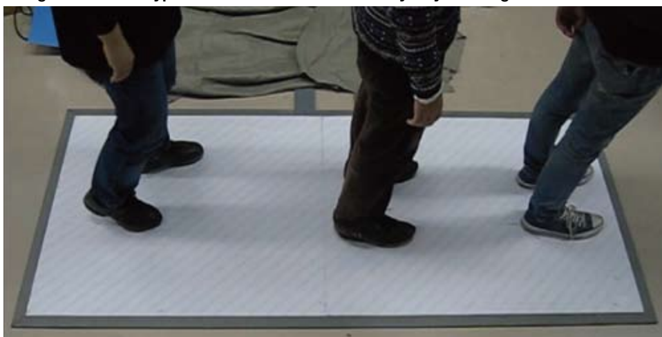
■ Figure 2: Sheet-type sensor covered with ordinary vinyl flooring material.
