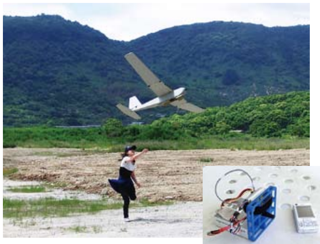
■ Photo 1: Launching a small-scale drone by hand, and a close-up view of the on-board wireless relay
